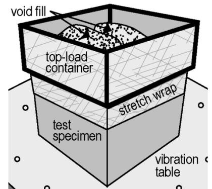
The **Top Load Apparatus** required for the vibration testing of **Type D, Type E, Type F and Type H** packaged-products is detailed below
