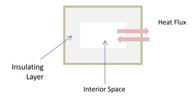
If the interior space has a temperature higher than the exterior air temperature, heat passes out of the container. If the interior space has a temperature lower than the exterior heat passes into the interior from the outside. The Insulating Layer moderates the rate at which this happens. More insulation equals a lower rate of heat flux. Insulation simply works to slow heat exchange processes to keep interior temperature from changing too fast.
