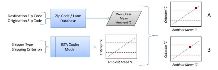
Inputting the geographic data yields an output of the Worst Case data expected for the hottest of summer to the coldest of winter. An internal programmatic process that finds the closest matching lane combination from the ISTA lane database, and returns the mean temperature for that closest match.
