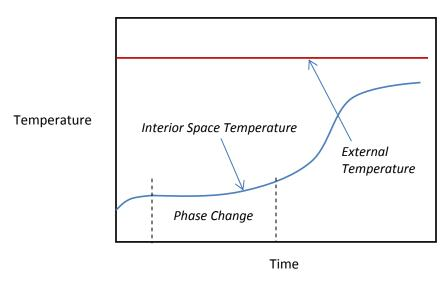
There is an initial rise in temperature as the phase change material approaches its melting point. As it melts, temperature is stabilized; the incoming heat is absorbed by the material without a change in temperature.
