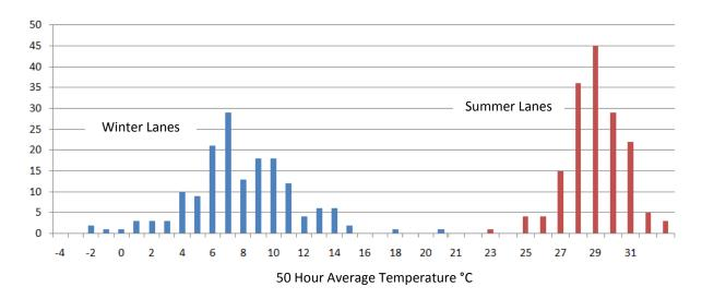
As we will see from the analysis in subsequent sections, the Winter Lanes in the "low tail end" of the distribution will affect the performance of Insulated Shipping Containers in a non-linear way when temperatures drop below certain limits.
