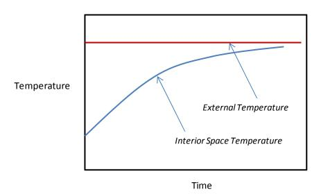
As time progresses, the internal temperature becomes asymptotically closer to the external temperature.
