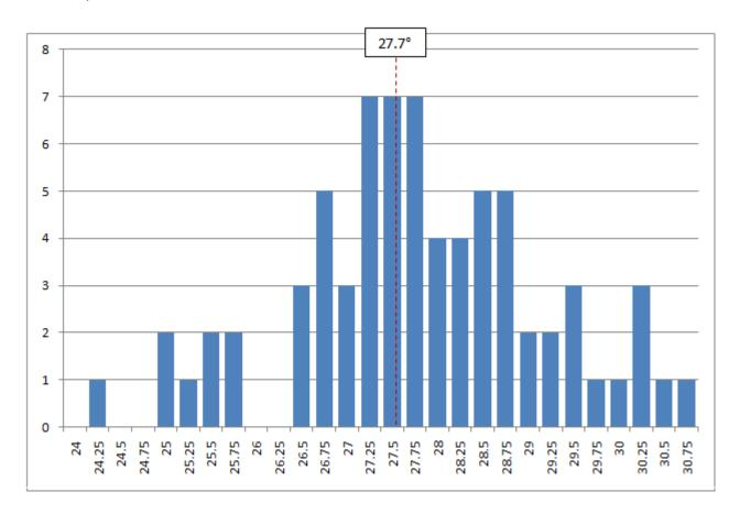
The vertical axis is frequency and the horizontal axis is average 72 hour temperature for lanes. The dashed red line represents the average for the 7E profile (a type of "grand mean").
