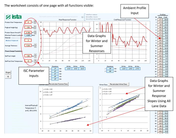
ISC Parameter Inputs are performed by "spinners" which gradually increment or decrement values. Ambient profiles can be input by clicking buttons for either the ISTA 7E standard profile or the well-known Amgen profile. Users can also input their own ambient profiles by data entry into the ambient profile columns shown on the right.
