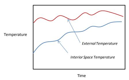
The thicker the insulation, generally, the less impact exterior oscillations will have on the profile of the Interior Space Temperature. In a very well insulated container, the interior temperature profile would look much more like the first graph.
